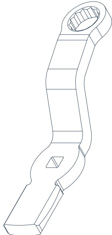
→ Changing a brake cylinder without needing to completely dismantle the entire wheel: The new impact wrench from PE and HAZET makes for faster and simpler work. For repairs in record times.
